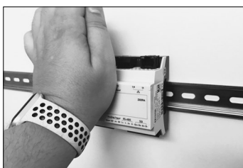
Press device onto top-hat rail
