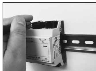
Press device onto top-hat rail
