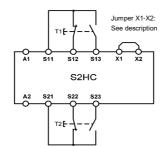
Fig. 4: Wiring of the S2HC with a 2-hand push
