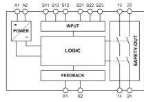
Fig. 1 Block diagram S2HC
