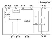
Fig. 1 Block diagram SR2C
