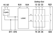
Fig. 1 Block diagram SREC
